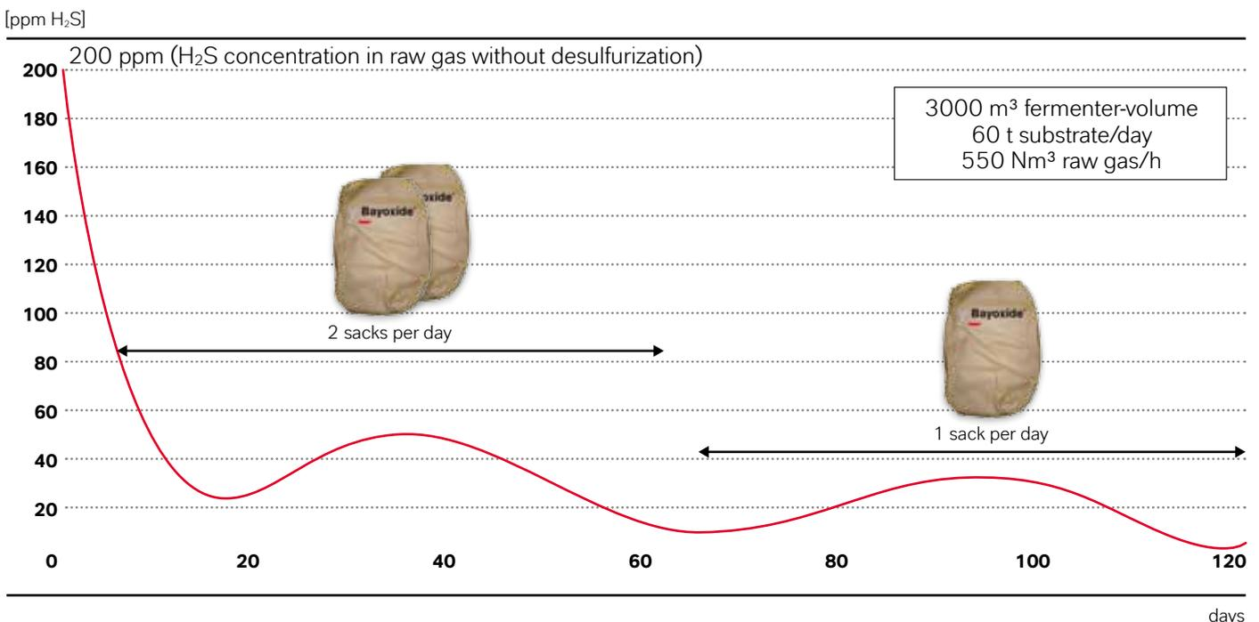
Reduction of H<sub>2</sub>S concentration during desulfurization with Bayoxide® E 16
