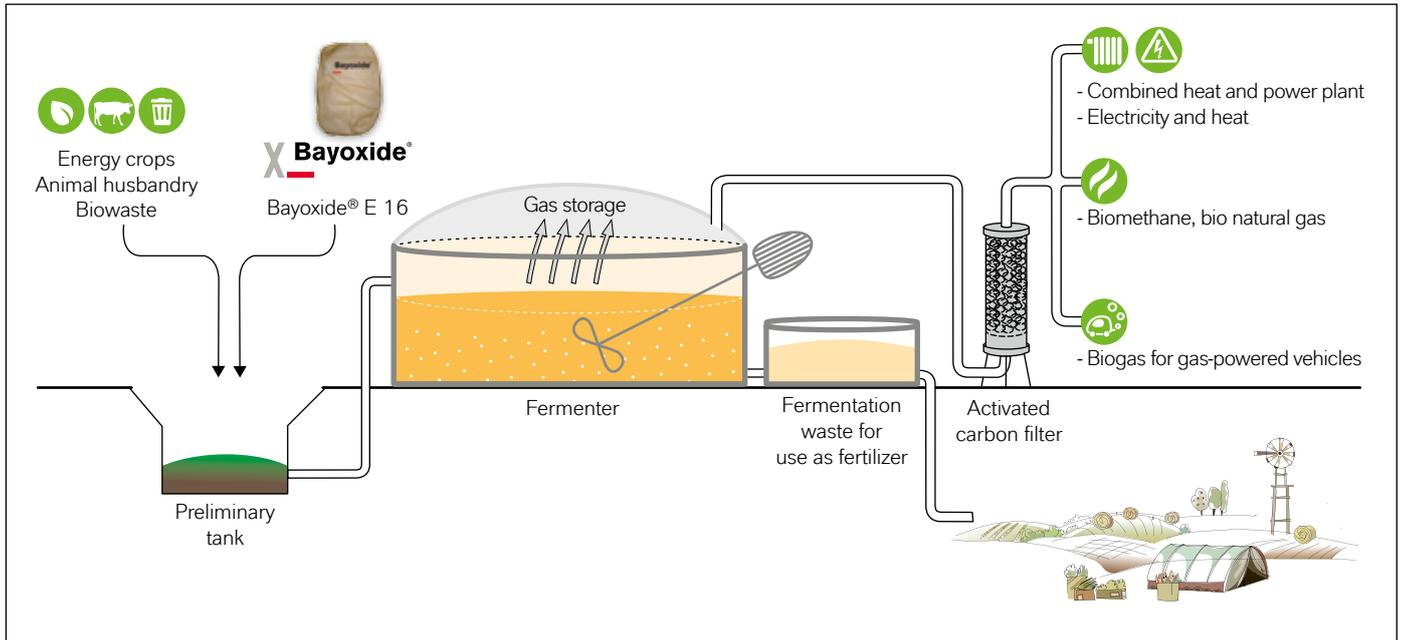
Diagram showing how Bayoxide® E 16 is used
