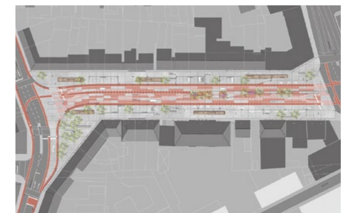
■ The layout shows the cast-in-situ concrete fields, integrally colored with varying pigment concentrations – a nod to the original rose beds.
